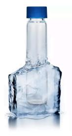
As a rule, the sample has a higher coefficient of thermal expansion than the borosilicate glass of the laboratory vial. Therefore, the vial should only be filled to  $\frac{2}{3}$ , maximum  $\frac{3}{4}$  of the possible volume so that the liquid has room to expand. Otherwise, the closed vial may burst due to the increasing pressure inside.
